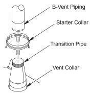
Figure 9 - Installing Transition Pipe and Starter Collar
